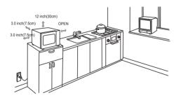
A minimum clearance of 3.0 inches (7.5cm) is required between the oven and any adjacent walls. One side must be open.
